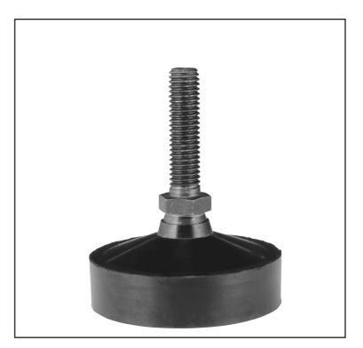
LMS attenuated levelers are designed for leveling, aligning and isolating sensitive electronic manufacturing equipment. LMS Series levelers feature over .5" of neoprene elastomer bonded to the bottom of the leveler to provide shock-attenuated, non-skid support.
