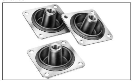
Barry Controls Multiaxis Mounts are designed for low-frequency vibration isolation. These all-attitude isolators provide effective vibration protection in all directions and are available in either square or diamond configurations. Snubbing washers provide an interlocking system of metal fasteners which act to prevent damage from overload or excessive shock impact.
