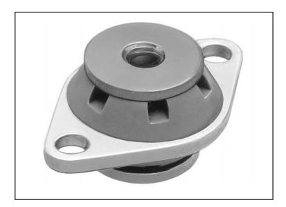
Barry E Series Mounts are designed for optimum shock and vibration isolation of lightweight electronic equipment, where space is a concern. E-Mounts are ideal for isolation where random vibration environments occur, such as in military or commercial aircraft applications.
