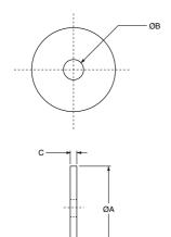
The use of snubbing washers is recommended to ensure proper static and dynamic loading of the isolator and retention of suspended equipment under severe shock environments.
