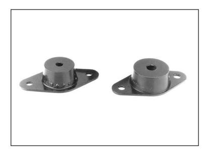
Barry HR Series mounts are best suited for isolation of diesel engines with five or less cylinders for on or off-highway applications. The standard neoprene elastomer provides resistance to oils and most solvents. Other elastomers are available, consult factory for more information.
